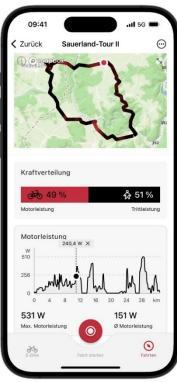
While the app displays the distribution of motor and pedal power in a bar chart, a line diagram illustrates the motor power. The graphs of all categories can be operated interactively and are synchronized with each other – they display their values at any point during the tour. (image rights: Brose)
